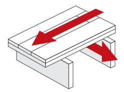
Additionally, nail (ring shank) or staple layers together on a minimum 12" grid pattern. Sheets should be glued to lumber subfloor using good quality
