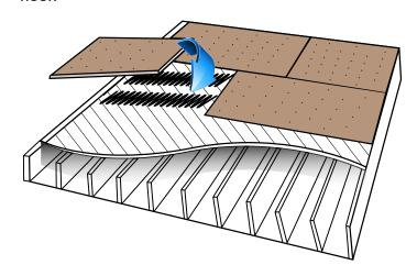
NOTE: Do not install in the same direction as existing floor.
