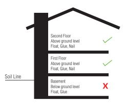
Installation of cabinets on top of nail-down and/ or glue down floors can contribute to squeaking or objectionable noises in floor.
