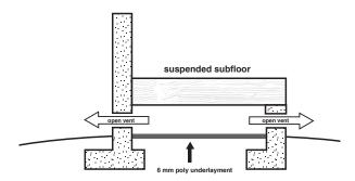
Size of available vents should equal to 1.5% of the square footage within the crawl space. Relative humidity should be consistent with interior of home.
